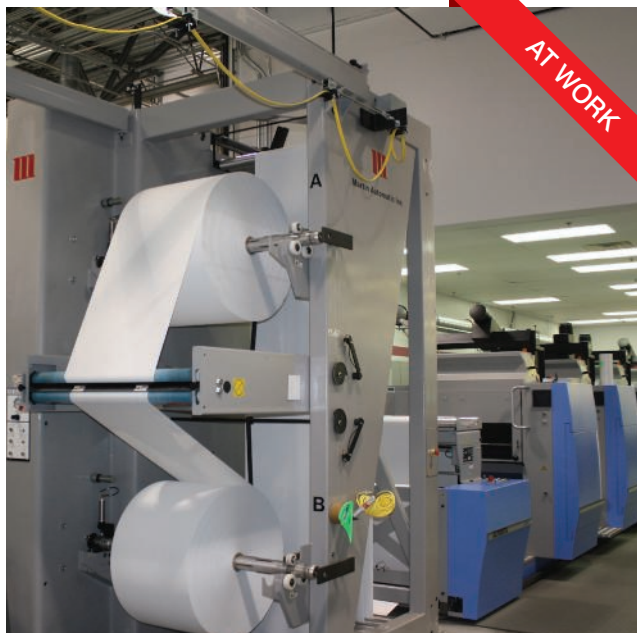
At Keller Crescent, a Martin Automatic ECP splicer is increasing productivity on a Muller Martini Alprinta press.
